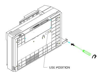
Figure 2-2 Securing the Shipping Bracket
